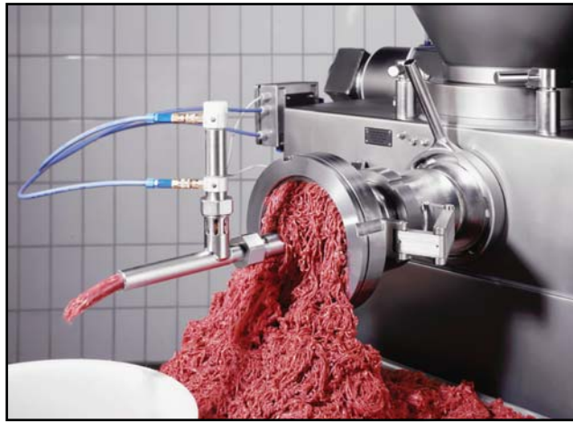
Automatic separation valve on separation attachment 801
